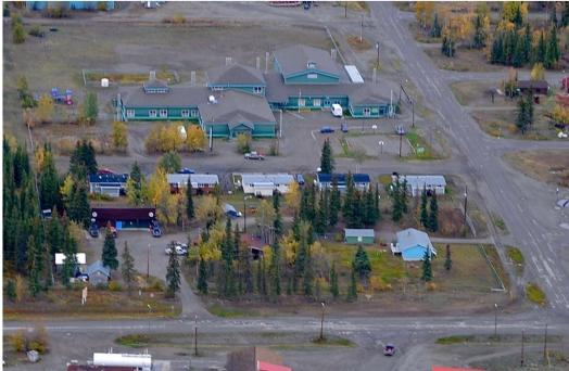
A challenging site with deep discontinuous warm permafrost. There was no reasonable alternative to thermosyphons for a structure the size of the school given the architects functional requirements
